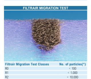
(\*) Number of particles larger than 10 microns per cubic meter counted on
